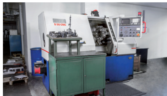
Lathe S 50 CNC d = 270 mm · l = 535 mm
