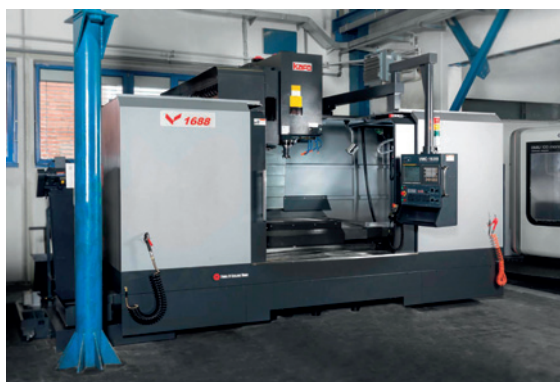
Vertical milling center KAFO VMC-1688 x = 1600 mm · y = 880 mm · z = 700 mm
