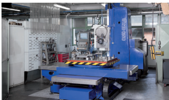
Horizontal boring machine - WH 10 CNC Table 1000 x 1120mm with rotation Travels (X = 1250mm, Y = 1000mm, Z = 900mm)
