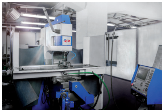
CNC milling machine FV 30 x = 760 mm · y = 380 mm · z = 152 mm
