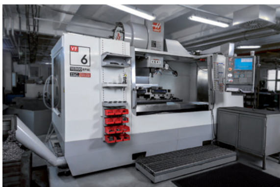
HAAS VF-6 x = 1626 mm · y = 813 mm · z = 762 mm
