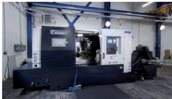
Lathe GOODWAY GS-4000 d = 620 mm · l = 600 mm
