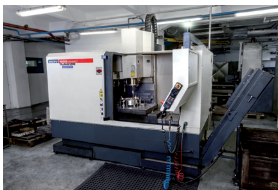
Vertical milling center MCFV 1050 x = 1020 mm · y = 510 mm · z = 525 mm
