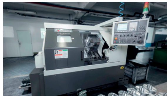
Lathe GOODWAY GA-2600 d = 606 mm · l = 530 mm
