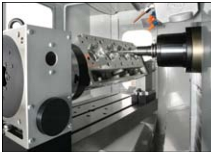
The ES-5-4T with 4th-axis rotating table is perfect for complex operations like cylinder head porting. Simply mount a rotary table and fixture to the T-slot table for full 5-axis machining capability.
